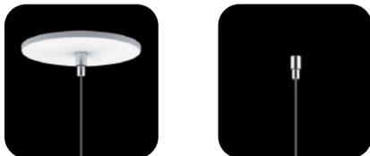
5" diameter power feed canopy and no canopy on the non-power feed side. Minimal aesthetic. Requires a 1/4-20 stud securely attached to ceiling. Works well with continuous runs where the power can be carried inside the fixture.
