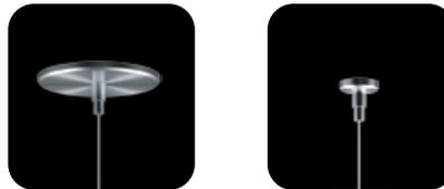
4" diameter machined power feed and 1-1/4" diameter machined non-power feed canopy. Offers minimal ceiling treatment while maintaining the ability to cover mistakes. Requires a 1/4-20 stud securely fastened to the ceiling. Mill, anodized, and powder coat finishes available.
