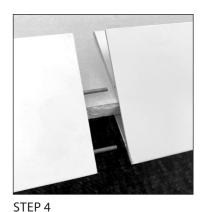
Slide alignment pins into extrusion leaving about 1" protruding.
