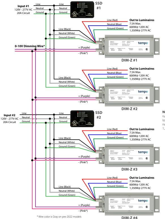
**NOTE:** No limit to number of runs from output of DIM-Z as long as total wattage does not exceed 600W@ 120V or 1,350W@ 277V.
