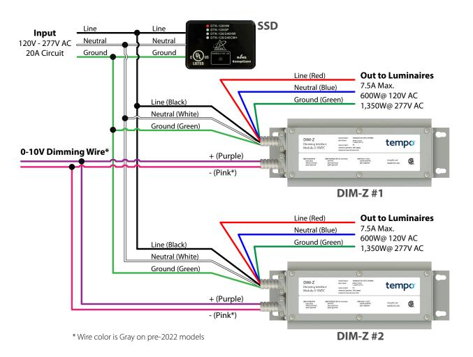
**NOTE:** No limit to number of runs from output of DIM-Z as long as total wattage does not exceed 600W@ 120V or 1,350W@ 277V.
