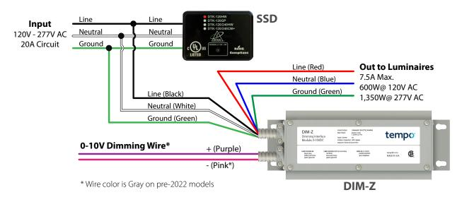
NOTE: No limit to number of runs from output of DIM-Z as long as total wattage does not exceed 600W@ 120V or 1,350W@ 277V.
